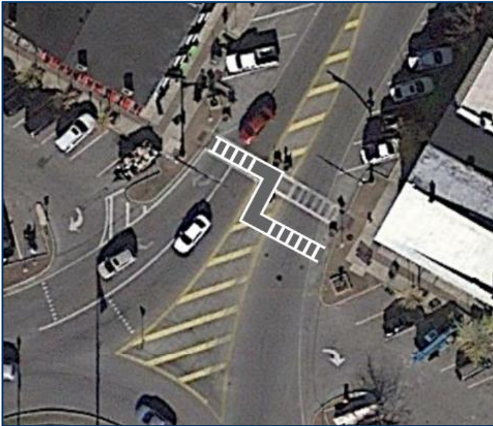
Figure 6: Zig Zag Crosswalk
