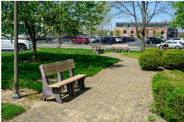
Benches at Bruckner Park are located well for clearance and pulling alongside them. The benches themselves should be replaced with accessible benches.
